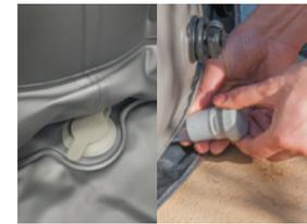
13) Check that the drain plug is closed properly.
